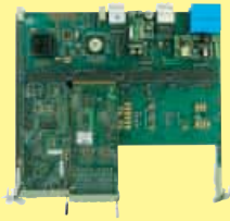
AdvancedTCA ® carrier board with AdvancedMC ™ modules
